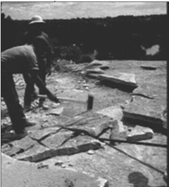
These men are using hammers and picks to break off slabs of limestone from a riverbank outcropping.
