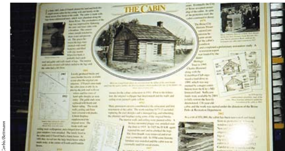
Porcelain enamel panels are durable and stable but expensive to produce.
