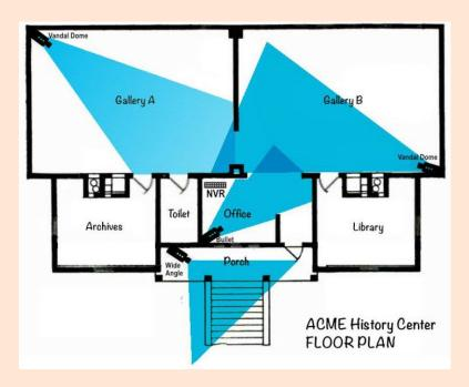
Floor plans for security systems should show placement of components. A key should be provided.
