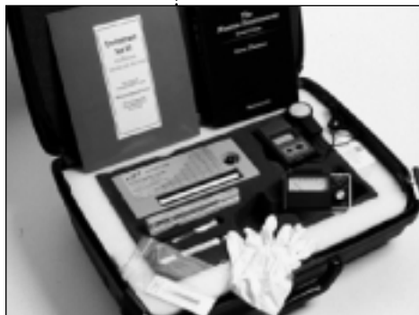
Figure 2, above. Environmental Test Kit. The kit includes instruments for measuring visible and UV light, a psychrometer for measuring RH, several inexpensive monitoring tools (see figure 3), and a manual.
