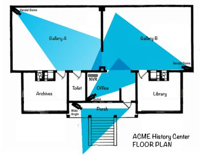
**Floor plans for security systems** should show placement of components. A key should be provided.
